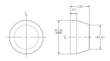
SEAVEY / COMTECH replacement feed windows. Made of White PVC, .020 thick and UV Stable for long term outdoor exposure. These units do not fit Chaparral feeds. PART#- SV-FWU-8538-35
